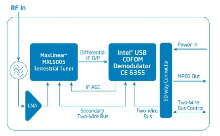
The Intel CE 9525 DVB-T TNIM reference design kit is supplied with only a single +5 volt supply, since all other power rails are generated onboard. The Intel CE 9525 DVB-T reference design frontend solution is optimized for real in-field terrestrial environmental conditions. Supplied as a tested and characterized application board, the reference design provides a reliable, fast time-to-market DVB-T digital front-end solution.
