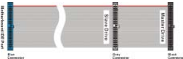
Figure 2-8. Ultra DMA 66 Ribbon Cable Outline
