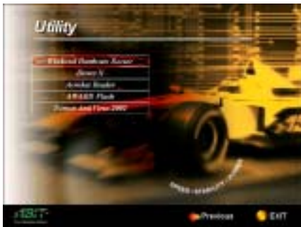
Step 2: Click "Winbond Hardware Monitor" button to start install the hardware monitor system utility.
